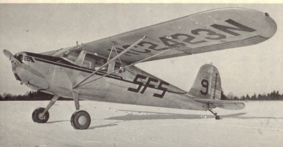
The 85 h.p. Cessna 140, put on the market after WW II, drew heavily on the prewar Luscombe for structural and aerodynamic features. Its most interesting innovation was the single-leg spring steel landing gear that had been developed by Steve Wittman for use on his racing planes in the mid-1930's. Photos by the author
