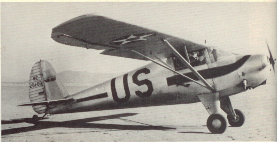
The Luscombe 8C of 1940, identical to the 65 h.p. 8A model except for fuel-injection Continental A75 engine. Military markings do not mean that Luscombes were in the Army. The big U.S. on the fuselage and the star on the wing were required for general aviation aircraft flying near the West Coast after Pearl Harbor.
